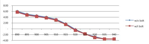
•SECURE HT reads same, regardless of whether it is fastened with metal bolt in two holes (located on center of both ends) or not. Stainless steel M3 bolt with round head is best fit for SECURE.
