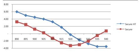
•SECURE HT reads up to 5.5 meters on metal, same as original SECURE. Though not best performing among similar size tags, its performance is most stable and consistent, as its slow and gentle slope of sensitivity curve shows.
